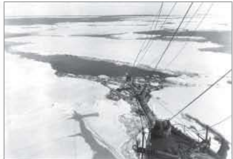
The Endurance cuts through pack ice. The ship's hull was sheathed in greenheart, a durable wood that can withstand battering by ice.
